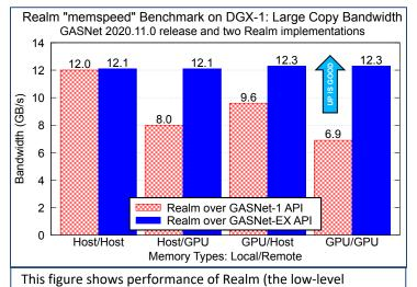
runtime of the Legion ST project) with their GASNet-1 ("then") and GASNet-EX ("now") backends. The latter uses many features new to GASNet-EX. These results show one benefit of using GASNet-EX features: performance of RMA involving GPU memory matches that of host memory RMA. See also SC21 poster: doi:10.25344/S4P306 Data courtesy of Sean Treichler of the Legion team
