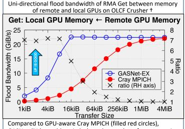
GASNet-EX (open blue circles) reaches peak performance using smaller transfers. Both implement RMA transfers involving GPU memory using ROCmRDMA (direct PCI peer-to-peer transfers) between the GPU and NIC. GASNet-EX has up to a 7.2x RMA flood bandwidth advantage (the ratio is plotted with Xs against the right-hand axis).
